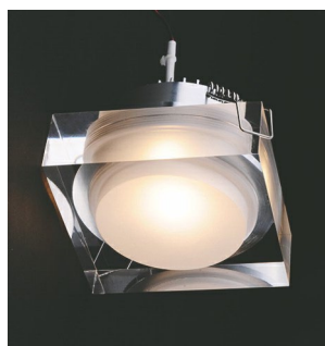
57387 LED quadratisch/starr 1 x LED CREE 13W 3000K 1400lm CRI >80
