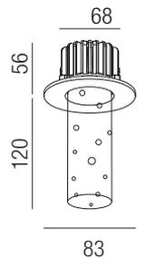
**Bubbles, IP20, 8W, 710lm, 3000K LED**
