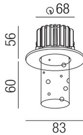
**Bubbles, IP20, 8W, 710lm, 3000K LED**
