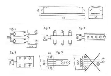
Electronic transformer is designed for halogen lamps, for voltage 12V.
