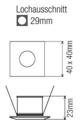
**Image Led flat**, LED 1W, 100lm, 3300K
