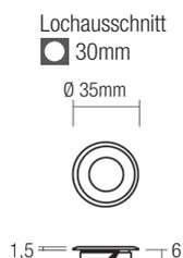
**Image Led flat**, LED 1W, 100lm, 3300K
