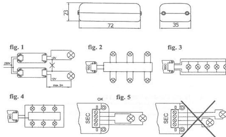
Electronic transformer is designed for halogen lamps, for voltage 12V.
